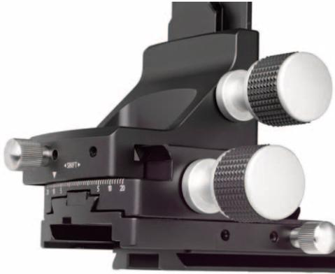
Let's take a look at the rear standard. It offers 40mm side shift using a quick slide and has a locking knob. The 12mm rise and 15mm fall is driven with a lockable fine gear. The optimum control of perspective enhances your creativity and quality possibilities for landscape, architecture and product photography.
