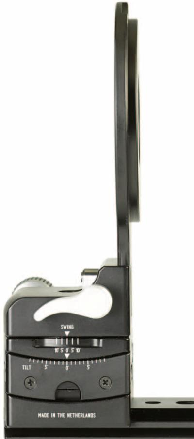
The front standard's tilt can be adjusted by 19°, the swing can do much more, even up to 360°. Needless to say, both by means of high precision fine gearing. These adjustments make it possible to change your selective sharpness plane, either to increase or to specify exactly your sharpness plane using Scheimpflug settings.
